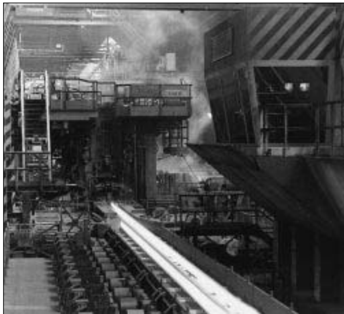
Fig. 3.14 The heaviest steel sections are produced by a hot-rolling process in which billets of steel are shaped by profiled rollers. This results in elements which are straight, parallel sided and of constant cross-section. These features must be taken into account by the designer when steel is used in building and the resulting restrictions in form accepted. (Photo: British Steel)
