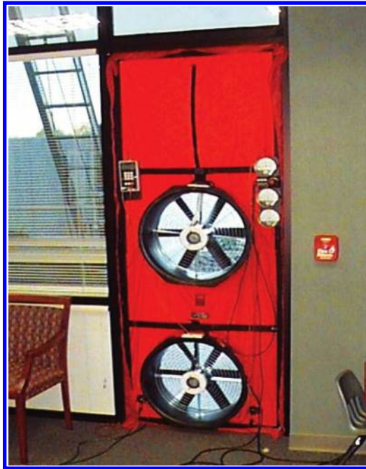
Color Figure 8.8 Blower door assembly.
