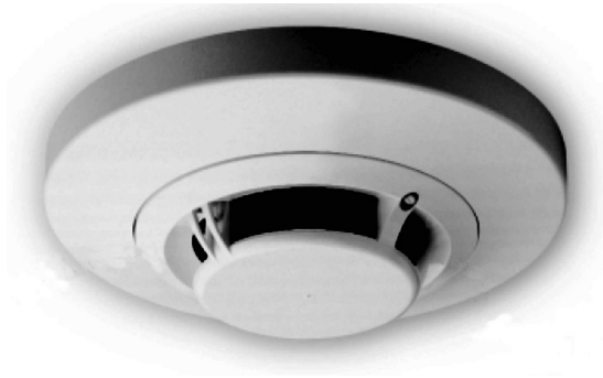
Figure 9.7 A multicriteria intelligent sensor, Acclimate that incorporates both thermal and photoelectric technologies that interact to maximize detection. Acclimate is a fire sensor with an onboard microprocessor with advanced software that makes adjustments to reduce false alarms. Source: System Sensor.
