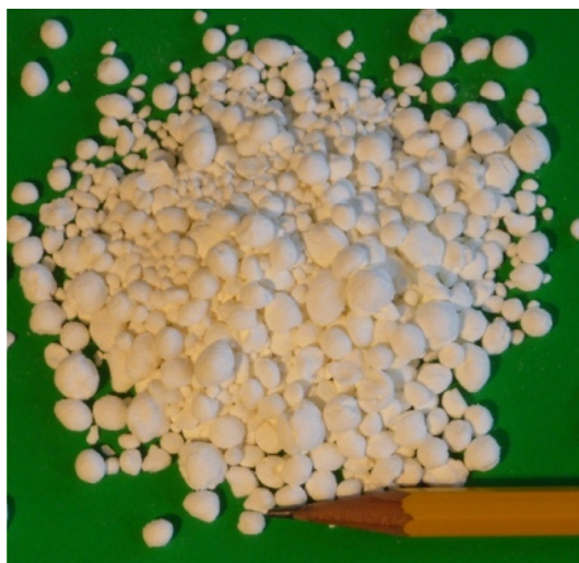
Fig. 8.15 The appearance of granulated form of native starch and glycerin.
