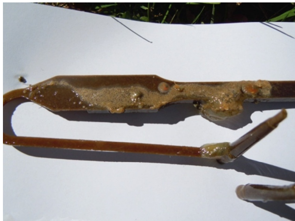
Fig. 7.1 Biological development on the surface of Flax/PLA biocomposite.
