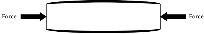
FIGURE 6.11 Compressive strength is the ability of a metal to resist crushing forces.
