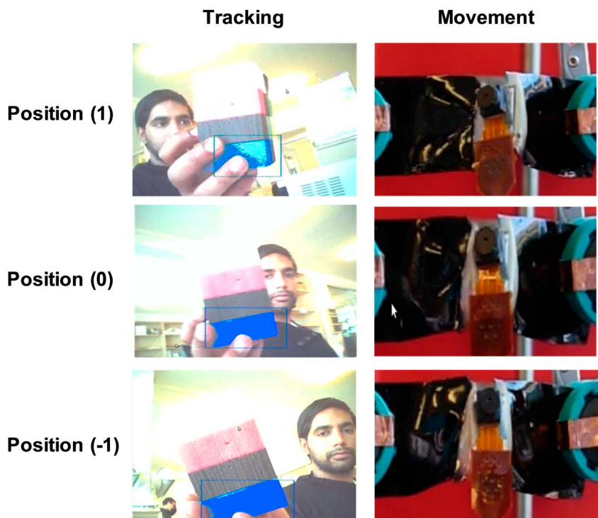
Figure 16.18 Resulting visual target tracking pictures (left) and corresponding device (right) in three different positions, (1), (0) and (-1).
