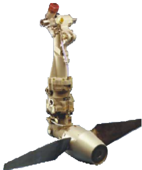
Figure 4.8. Hydraulic pump driven by dynamic air (image on the right used with the permission of Triumph Thermal Systems, Maryland Inc.) [EDU 13]
