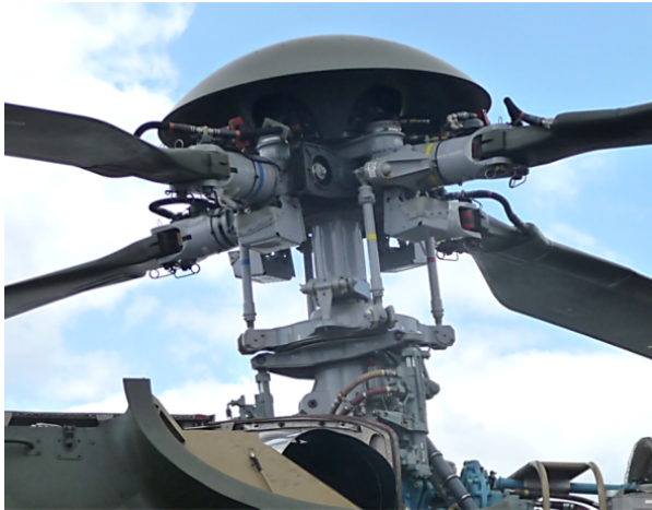
Figure 1.3. Swashplate actuation on an AS332 helicopter
