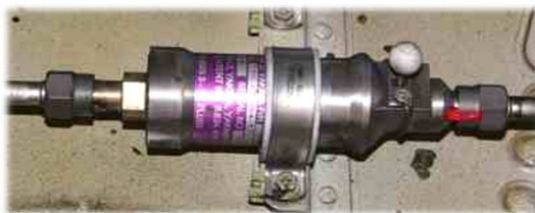
Figure 6.11. Hydraulic fuse (braking system of Boeing B737), (© Chris Brady)
