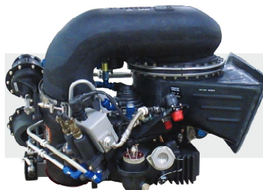
Figure 4.8. Hydraulic pump driven by dynamic air (image on the right used with the permission of Triumph Thermal Systems, Maryland Inc.) [EDU 13]
