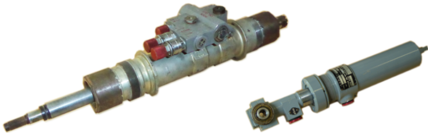
Figure 1.10. Jacottet-Leduc and Samm hydraulic assistance cylinders (Alouette III)
