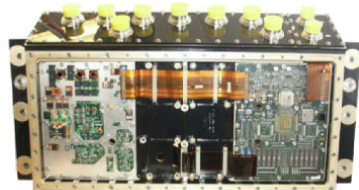
c) TVC EMA for strategic missile M51 (electronics from [GRA 04])
