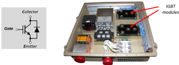
Figure 4.9. IGBT symbol and example of IGBT modules in the power drive electronics of a large civil aircraft EBHA. For a color version of this figure, see www.iste.co.uk/mare/aerospace2.zip
