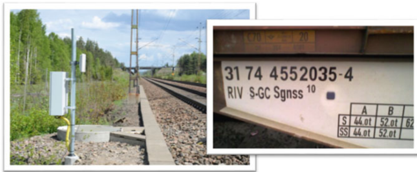
Fig. 3 RFID reader and tag attached to a wagon of the Swedish railways (Ivansson 2012)
