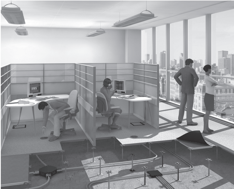
Figure 8.10 Raised access floors provide the flexibility to grant occupants individual control of the amount of air supplied through diffusers for their thermal comfort.
