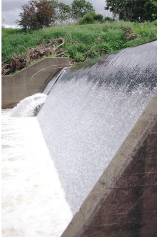
(B) Self-aeration down Jordan weir on Lockyer Creek (Qld, Australia) on March 2011 (shutter speed: 1/8,000 s).
