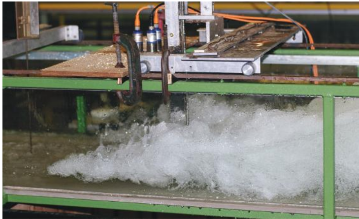
(B) Hydraulic jump in a rectangular channel ( V_1/\sqrt{g \times d_1} = 6.5 , \rho_w \times V_1 \times d_1/\mu_w = 1.5 \text{ E} + 5 ) - Flow from left to right.
