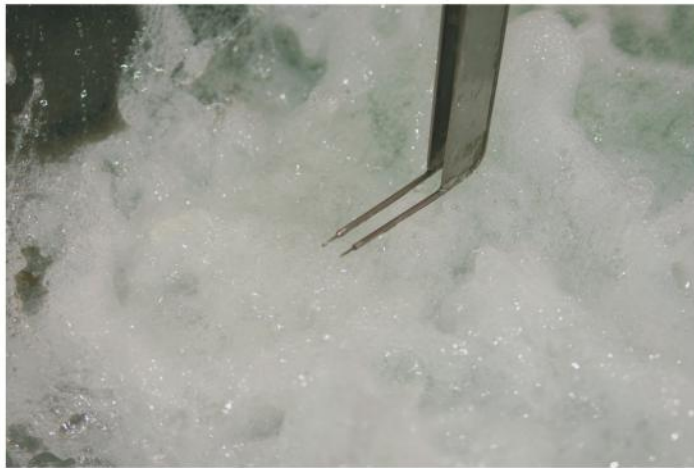
(B) Photograph of two single-tip conductivity probes side-by-side in a hydraulic jump ( Fr_1 = 6.6, \rho_w \times V_1 \times d_1/\mu_w = 8.6 E+4 ) – Flow from bottom left to top right.
