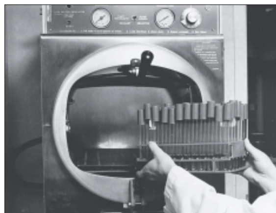
Figure 20.9 Tubes of media are sterilized in an autoclave for 20 to 30 minutes at 15 psi steam pressure.
