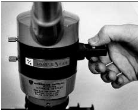
Figure 3.8 Some microscopes have an aperture viewing unit that can be used instead of a centering telescope for observing the orientation of the phase ring and annular ring.
