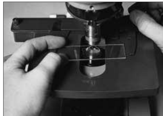
Figure 5.3 After calibration is completed, stage micrometer is replaced with slide for measurements.
