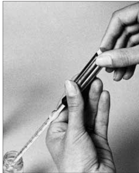
Figure 88.1 Using a mechanical suction device to draw up fluids into pipette
