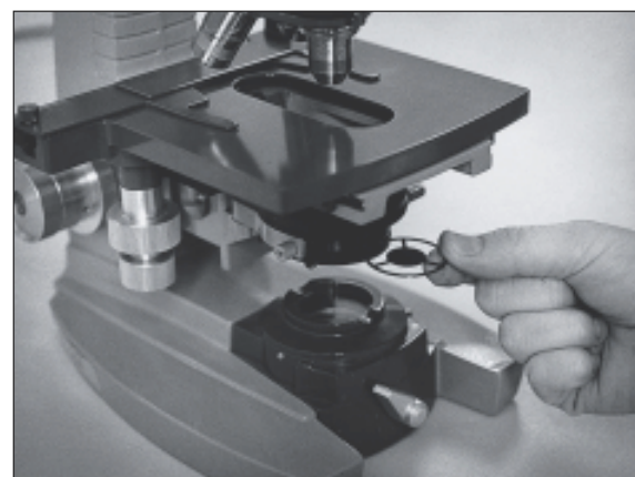
Figure 2.2 The insertion of a star diaphragm into the filter slot of the condenser will produce a dark field suitable for low magnifications.
