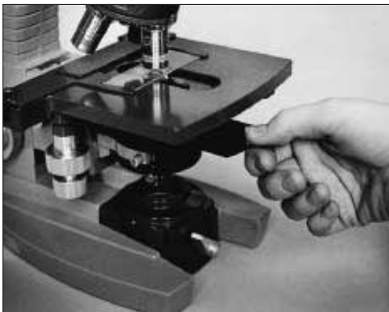
Figure 3.9 The annular stop on this American Optical microscope has the annular stop located on a slider. When pushed in, the annular stop is in position.
