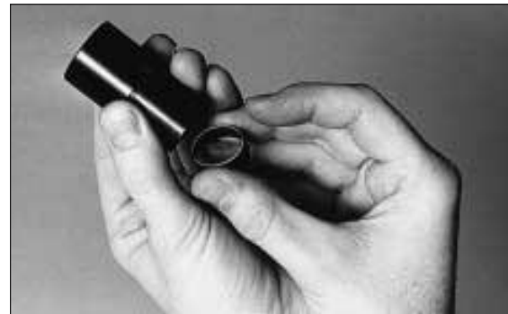
Figure 5.1 Ocular micrometer with retaining ring is inserted into base of eyepiece.
