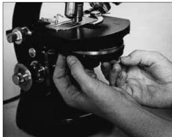
Figure 3.6 Alignment of the annulus and phase ring on this Zeiss microscope is achieved by adjusting the two knobs as shown.
