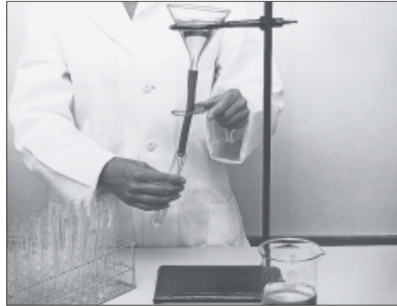
Figure 20.7 A glass funnel assembly and hose clamp are adequate for filling small batches of tubes.
