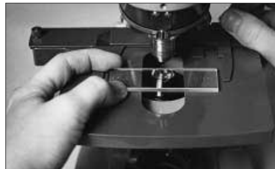
Figure 5.2 Stage micrometer is positioned by centering small glass disk over the light source.
