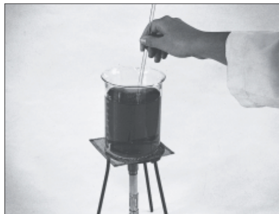
Figure 20.4 If medium contains agar, it must be brought to a boil to bring agar into solution.
