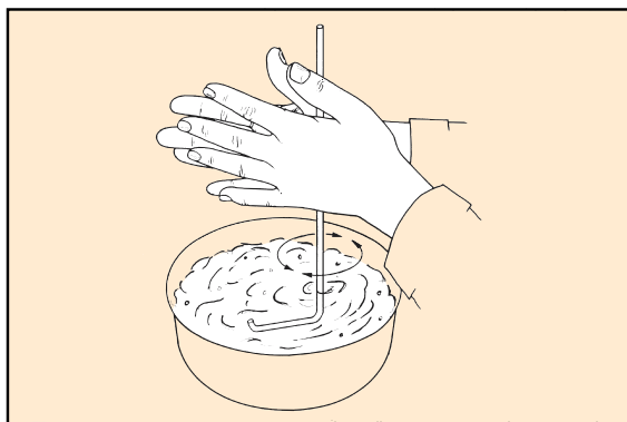
Figure 44.2 An alternative method of stirring utilizes an L-shaped glass stirring rod.
