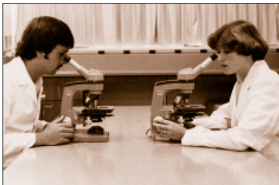
Figure 1.6 The microscope position on the right has the advantage of stage accessibility.
