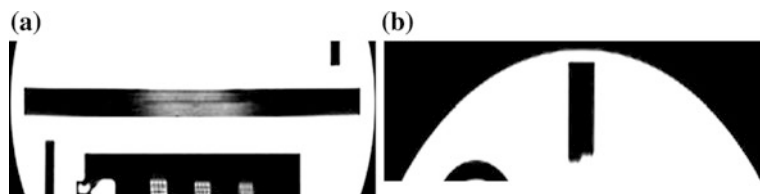
Fig. 10.7 a Slice thickness accuracy displayed in slice 1, located directly above resolution insert. b Slice position accuracy is evaluated by measuring the difference in the vertical bar lengths at the top of the phantom
