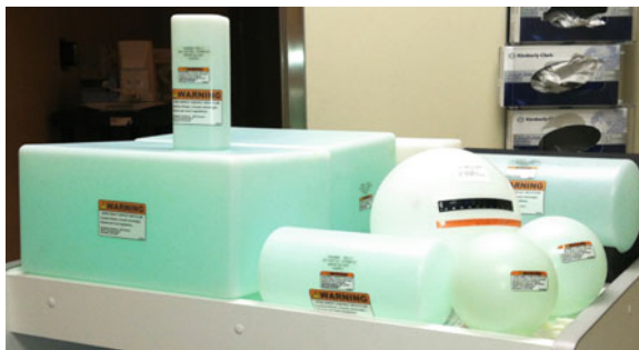
Fig. 10.1 A photograph showing several MRI loading phantoms provided with the General Electric Healthcare (Waukesha, WI) MRI system. Each vendor provides coil-specific loading phantoms
