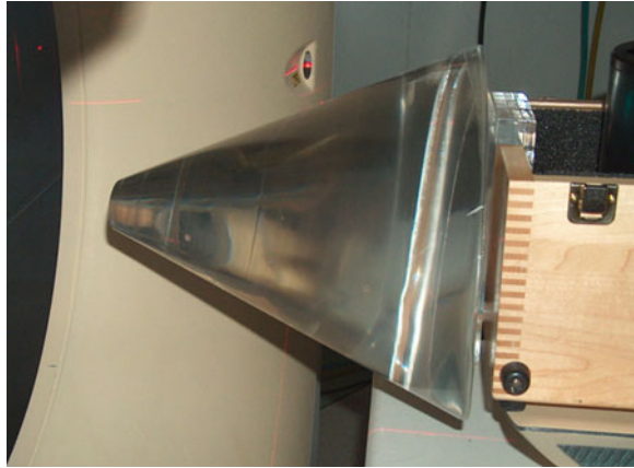
Fig. 7.9 Conical PMMA block for testing AEC response of the system when the patient size changes on the z-direction [96]
