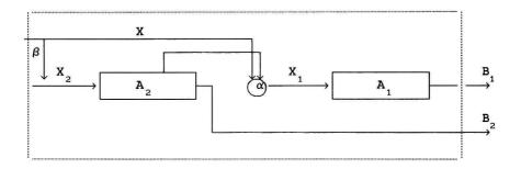
Different cascade connections of the automata  $\mathfrak{A}_1$  and  $\mathfrak{A}_2$  correspond to different triplets  $(X,\alpha,\beta)$ . For example, if we take a Cartesian product  $X_1\times X_2$  as X and define the mappings  $\alpha$  and  $\beta$  as corresponding projections  $\alpha(x,a_2)=\alpha((x_1,x_2),a_2)=x_1$ ,  $\beta(x)=\beta(x_1,x_2)=x_2$  where  $x=(x_1,x_2)\in X$ , then the cascade connection corresponding to such a triplet is a parallel connection of the automata.
