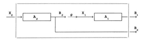
In the given construction an output signal of the automaton  $\mathfrak{A}_2$  is transformed into an input signal of the automaton  $\mathfrak{A}_1$  by means of the mapping  $\psi$ . The parallel (Cartesian product) and serial connections can be defined in this way also for the case of the semigroup automata.
