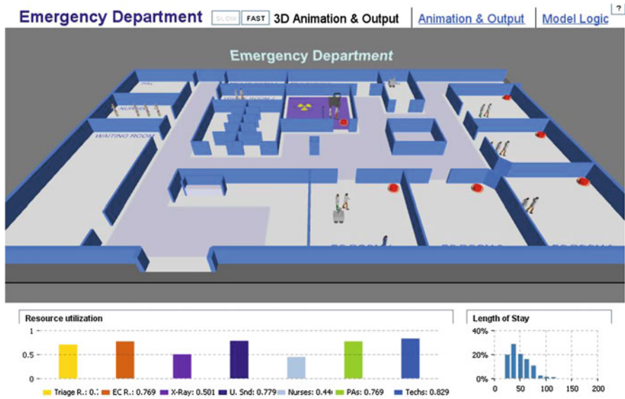
Figure 5: A discrete event simulation of an emergency department represents the entities involved and their attributes. It models resource utilization and also has queues where agents wait for finite resources. (Courtesy AnyLogic, All Rights Reserved)
