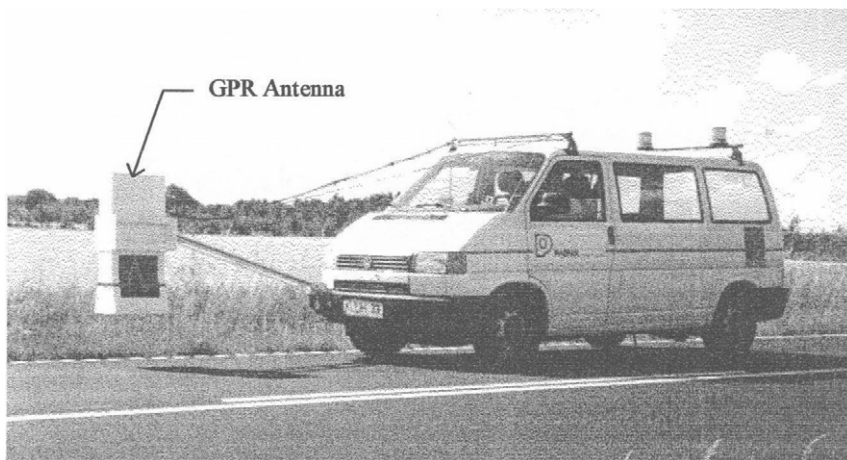
Fig. 2 - 1 GHz Horn Antenna GPR Equipment used for Airfield Runway Surveys
