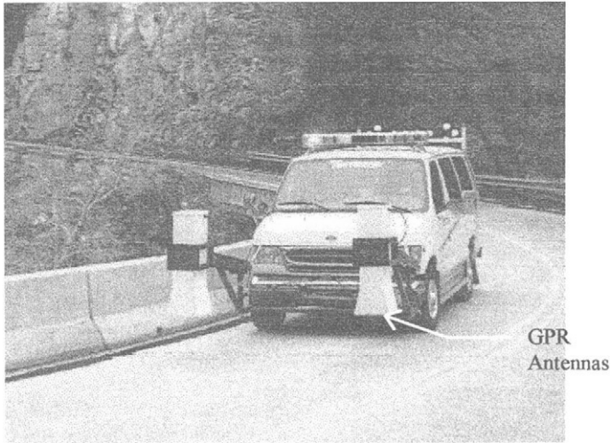
Fig. 1 - Field Setup of GPR Equipment
