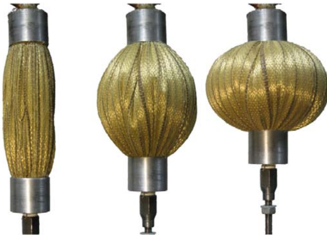
Fig. 2.1 Photograph of 3 contraction levels of the 1 st generation of PPAM.
