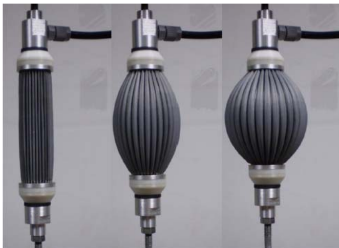
Fig. 2.3 Photograph of 3 contraction levels of the 3 rd generation of PPAM.
