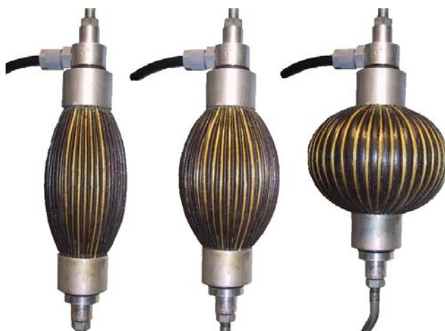
Fig. 2.2 Photograph of 3 contraction levels of the 2 nd generation of PPAM (used for Lucy).
