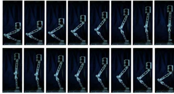
Fig. 1.24 A sequence of photos of a jumping motion of Chobino1D. The images were taken every 40ms with a high speed camera.
