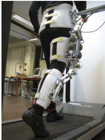
Fig. 1.15 Knee joint of the Altacro exoskeleton powered by PPAMs.
