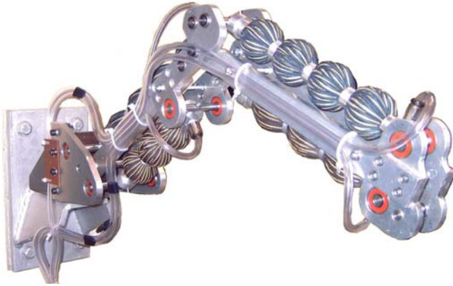
Fig. 1.25 Softarm actuated by PPAMs to study safe human-robot interaction.
