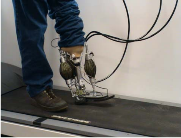
Fig. 1.16 IPPAM ankle-foot prosthesis powered by PPAMS.
