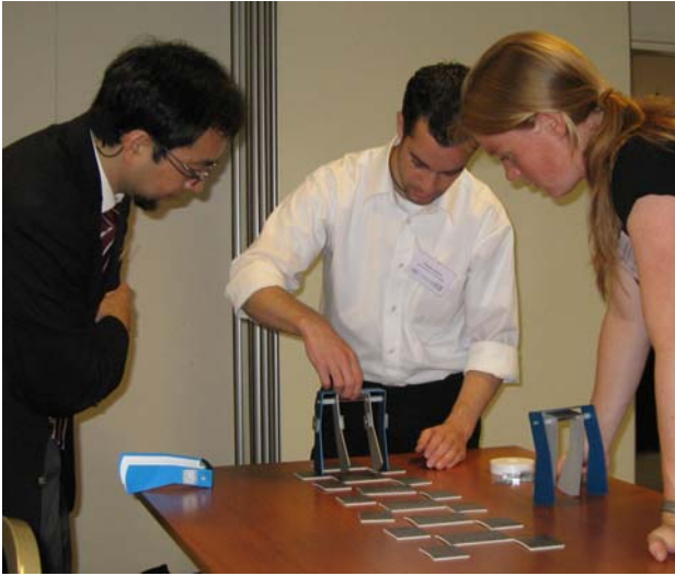
Fig. 1.26 Building and tuning the simple 2D passive dynamic ramp-walker Elvis during Dynamic Walking conference.
