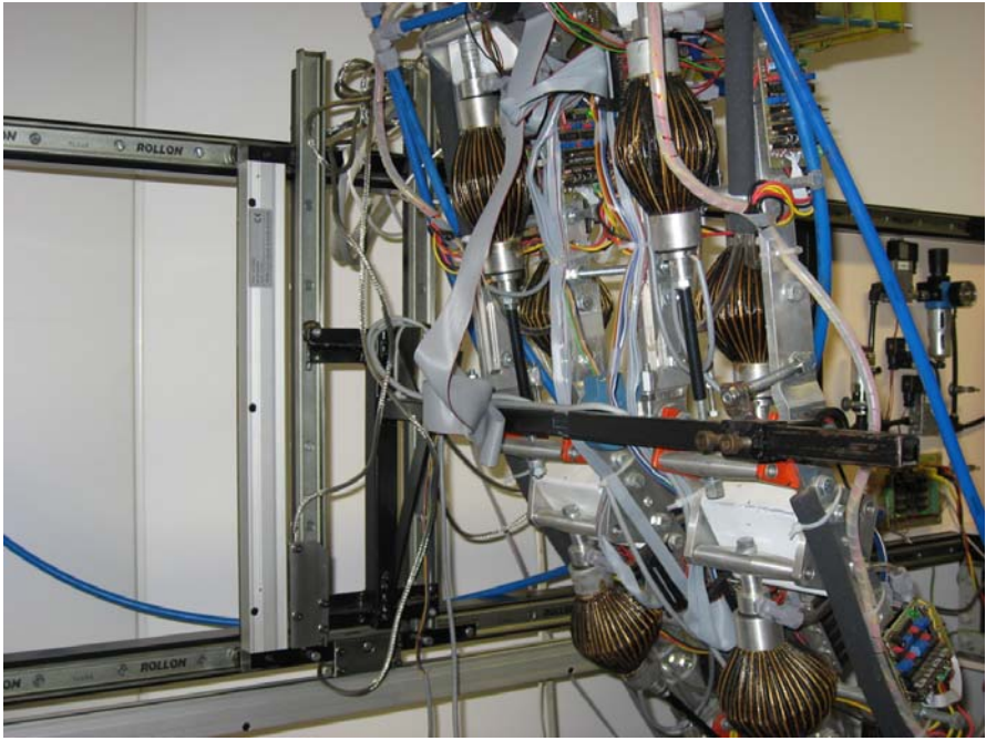
Fig. 2.23 Guiding mechanism consisting of two rails connected to the hip.
