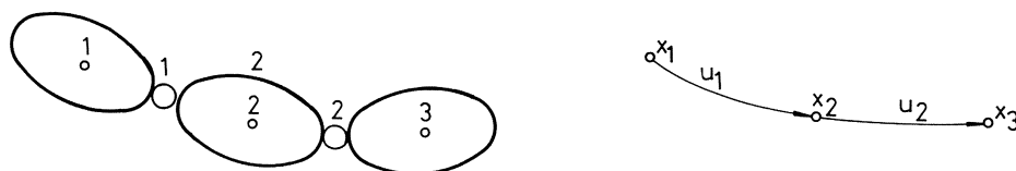
Fig. 12. Example of a system of bodies and the corresponding graph
