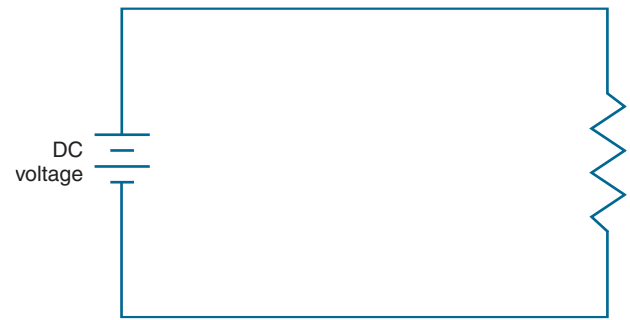
Figure 7-22 This simple circuit diagram shows a direct current source on the left and a resistor on the right.
