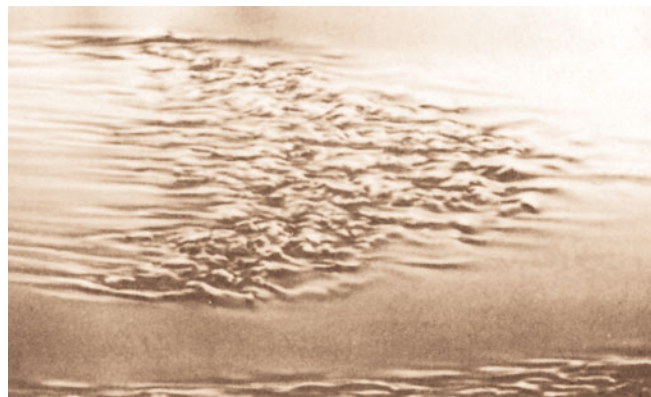
■ Figure 9.13 Turbulent spots and the transition from laminar to turbulent boundary layer flow on a flat plate. Flow from left to right. (Photograph courtesy of Brian Cantwell, Stanford University.)
