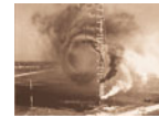
V3.5 Aircraft wing tip vortex, 108 Courtesy of NASA Dryden Flight Research Center
