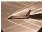
V11.11 Space shuttle oblique shocks, 658 © 2004 Gas Dynamics Laboratory, The Pennsylvania State University with a grant from the National Science Foundation
