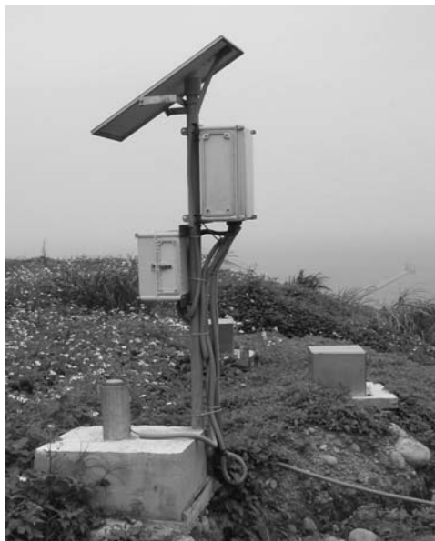
Figure 9.29 Solar-powered automated field data logging. (Courtesy of DECL, Taipei, Taiwan.)
