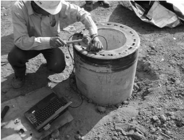
Figure 7.6 A spun-cast, pre-tensioned hollow cylinder concrete pile being tested for integrity. (Courtesy of DECL, Taipei, Taiwan.)
