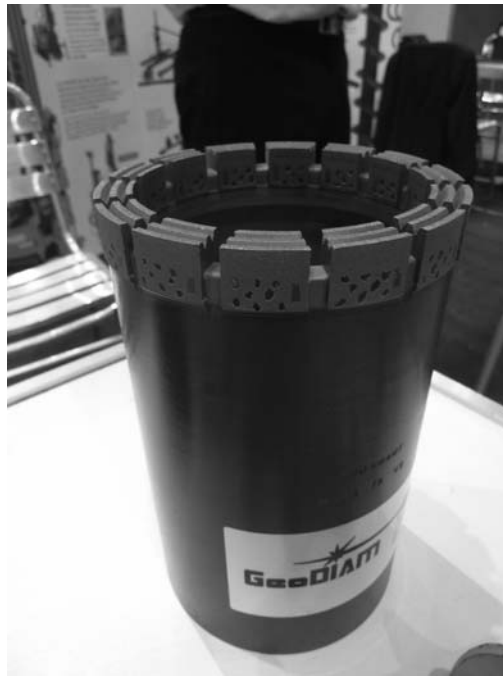
Figure 3.16 Photograph of a diamond coring bit. (Courtesy of An-Bin Huang, Hsinchu, Taiwan.)
