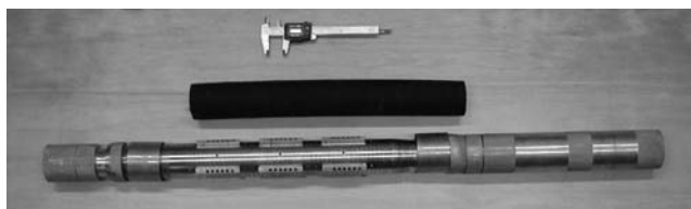
Figure 3.52 PBP with spring-loaded radial displacement sensors developed at National Chiao Tung University. (Courtesy of An-Bin Huang, Hsinchu, Taiwan.)
