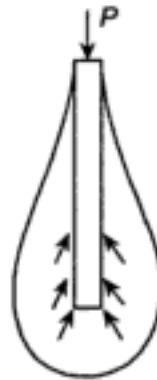
Fig. 9.3 Stress influence zone around piles.
