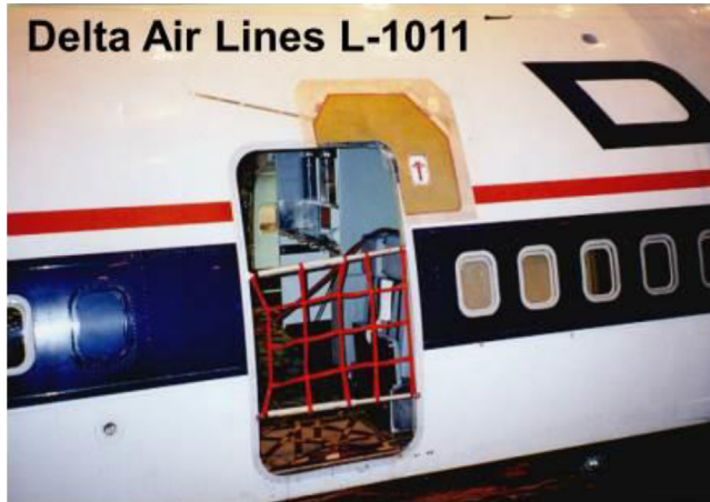
Figure 25.3 Bonded boron/epoxy composite doubler for repair of aluminum aircraft (Hart-Smith, 1999).
