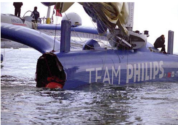
Figure 15.5 Team Phillips catamaran 2003 hits a freak wave with dire consequences, suffering a serious loss of function.
