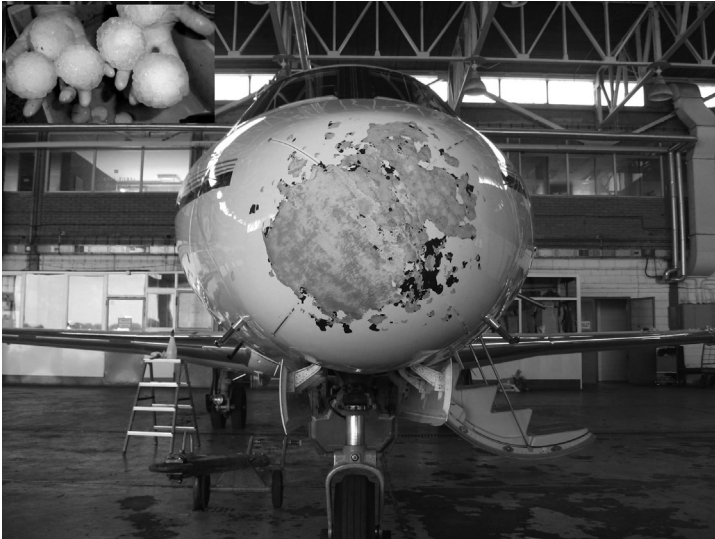
Figure 23.2 Hail strike-induced mechanical damage on nose cone of a Cessna 650 aeroplane. Courtesy Prince Aviation Company.
