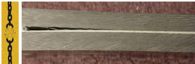
Figure 25.2 Bonded graphite/epoxy composite loaded to failure in mode I. Crack propagation is in the composite, the phase with the lowest fracture toughness in this structure.
