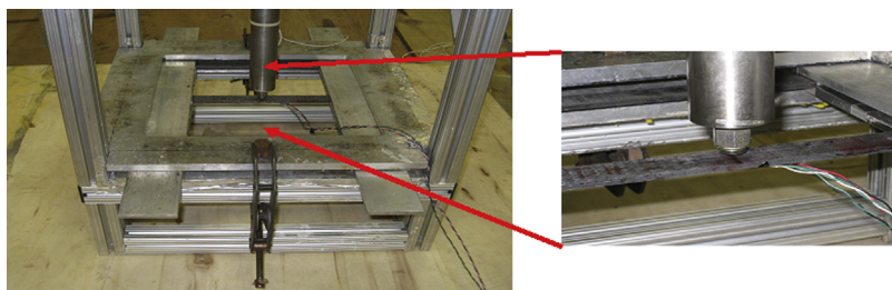
Figure 24.42 Test sample placed on impact test machine.
