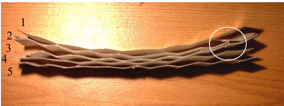
Figure 28.4 Edge view of the cold crushed layers with a tensile failure in layer 2 (ringed). Reprinted from Adams et al. (2014) , with kind permission from Springer Science and Business Media.
