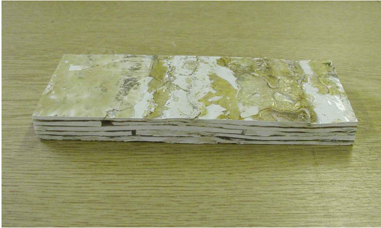
Figure 28.17 A multilayered plate manufactured from the bathroom component.
