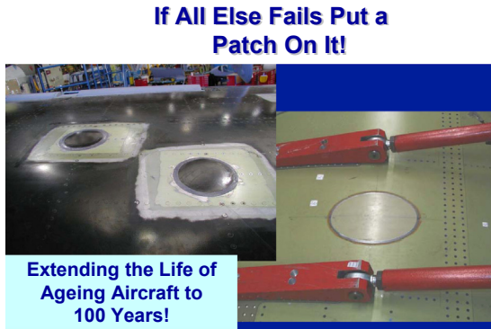
Figure 15.27 A glass fibre—epoxy patch over a fatigue crack in an aircraft aluminium alloy (Courtesy of Prof Endel Iarve).
