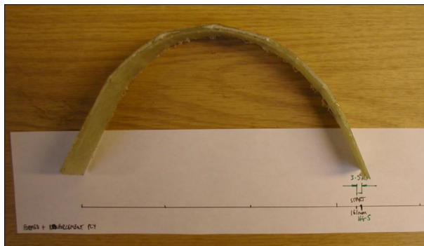
Figure 28.28 A reinforced F + H specimen after relaxation showing very little deflection.
