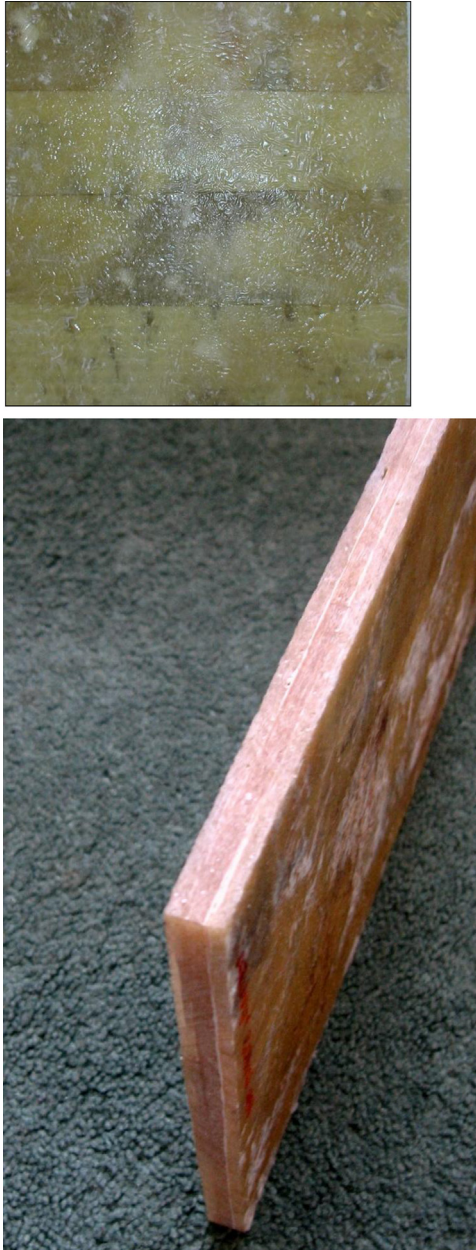
Figure 28.18 A multilayered plate manufactured from the boat hull.
