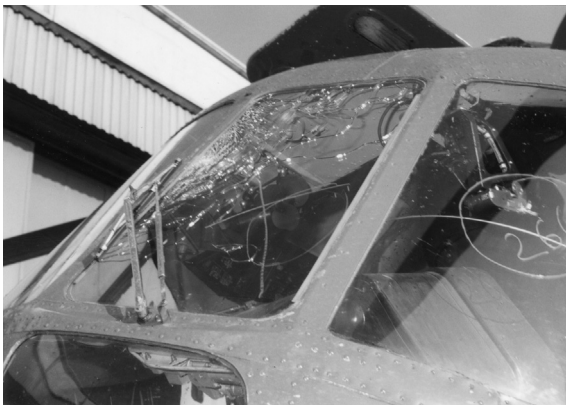
Figure 23.6 Ballistic damage to helicopter's windshield. Courtesy Moma Stanojlovic Company.
