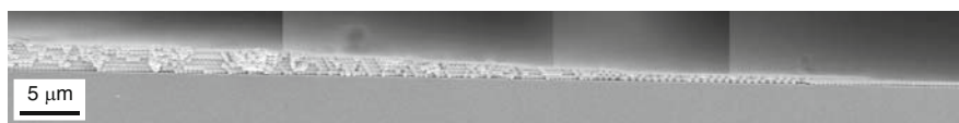
Fig. 4.4 SEM image of a cross section of the beginning of the assembled colloidal crystal film to illustrate the growth of multiple layers. Reprinted from Ref. 15 with permission. © 2008 Institute of Electrical and Electronics Engineers
