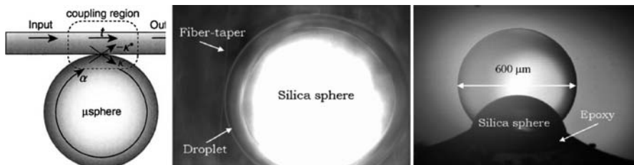
Fig. 17.11 Left : Outline of fiber taper coupling scheme to microsphere resonator. Reproduced from Ref. 33. Right : Fiber taper coupling configuration for liquid embedded microdroplet. Reprinted from Ref. 35 with permission. © 2008 Optical Society of America
