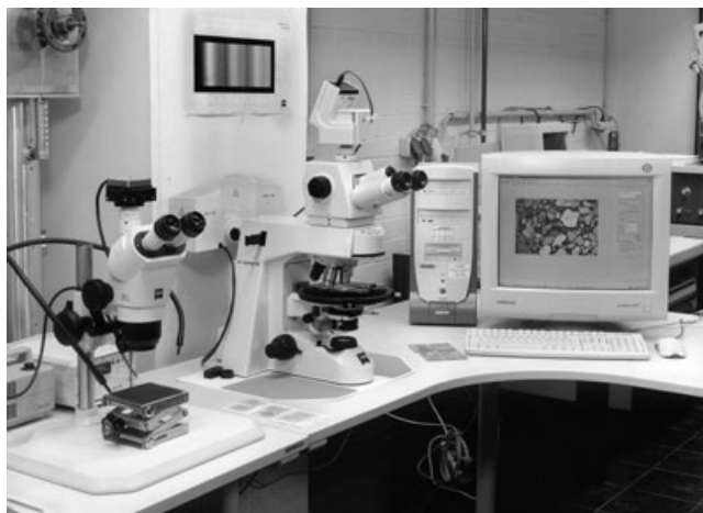
9.1 Standard equipment for the petrography of concrete comprises a stereo microscope and a petrographic (polarizing) microscope for thin section analysis. Modern systems allow the acquisition of photomicrographs via a digital camera. Digital image analysis software enables the user to retrieve quantitative data from some of the textural attributes.
