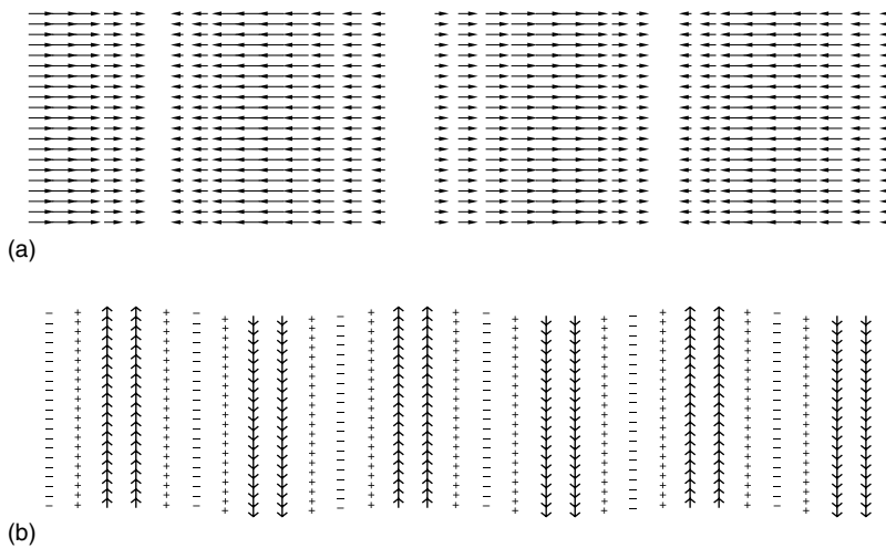
FIGURE 5.22 Simulation of plane waves: (a) pressure wave; (b) shear wave.
