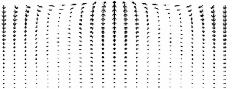
FIGURE 6.1 Simulation of Rayleigh wave in a semi-infinite medium.
