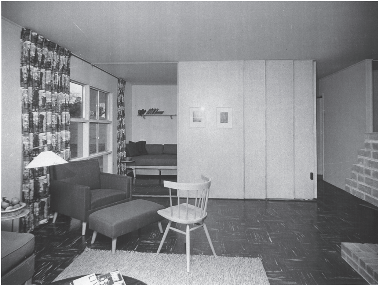
A sliding wall in the living room of a house in Levittown, Pennsylvania. The wall can be slid closed on a track to create a private guest room or opened to include the space in the living room. Courtesy of Bucks County Free Library, Levittown Branch.
