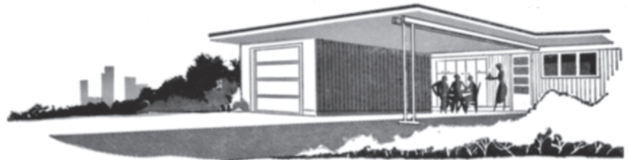
Instead of a double garage, this house has a carport and a single garage. The carport also serves as a covered outdoor living area. Storage space is provided in one wall of the carport.
