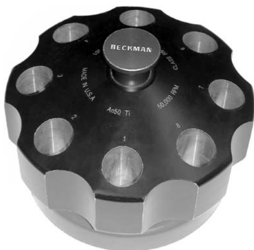
Fig. 2.5. Eight-hole analytical rotor made of titanium by Beckman-Coulter
