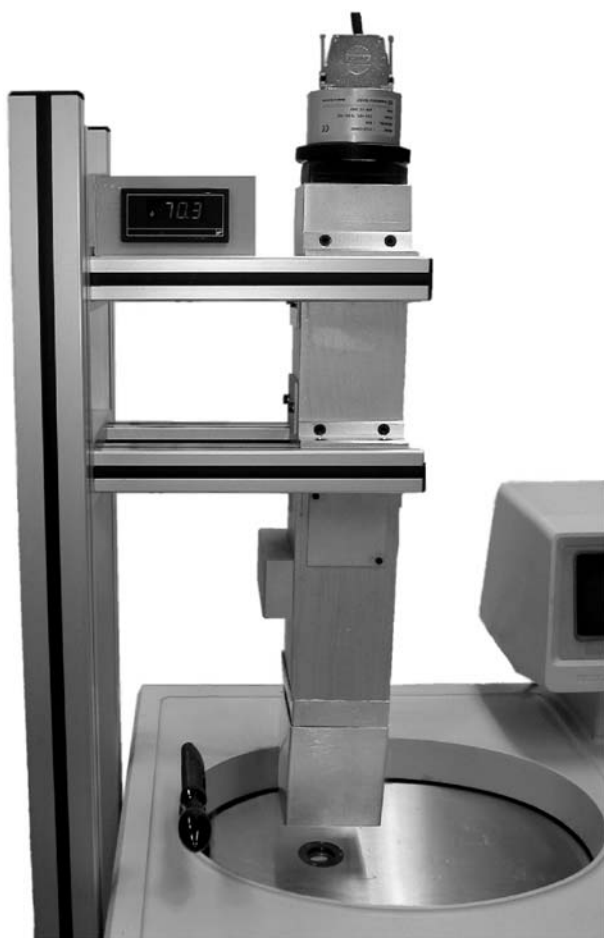
Fig. 2.4. Photograph of the physical Schlieren optics multiplexer setup of a modified Optima XL realized in the AUC laboratory at BASF
