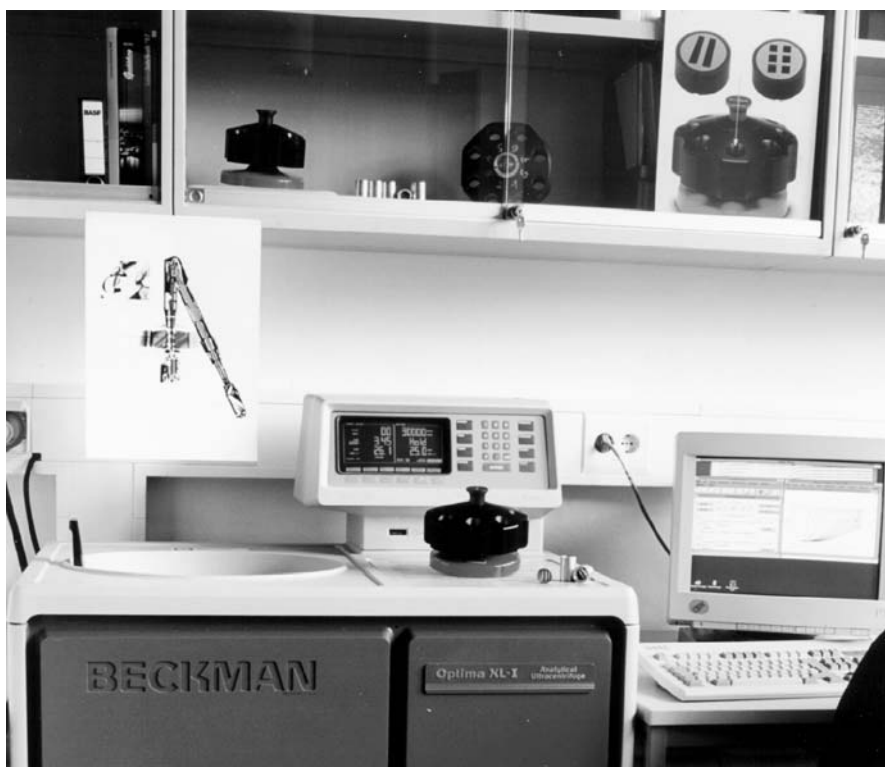
Fig. 2.2. Modern analytical ultracentrifuge Optima XL-A/I produced by Beckman-Coulter
