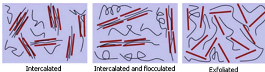
Fig. 2 Schematic representation of three types of polymer/clay nanocomposites, adapted from [25]
