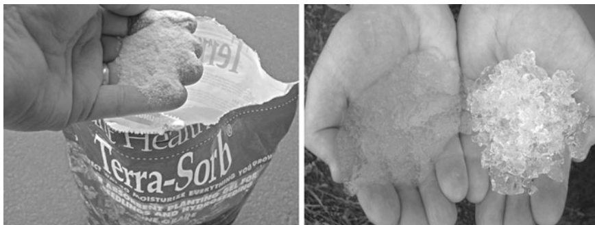
Fig. 10 Hydrophilic gels, commonly known as hydrogels, are dry crystals that can absorb many times their own weight in water. With permission from Ref. [156]. Rocky Mountain Research Station
