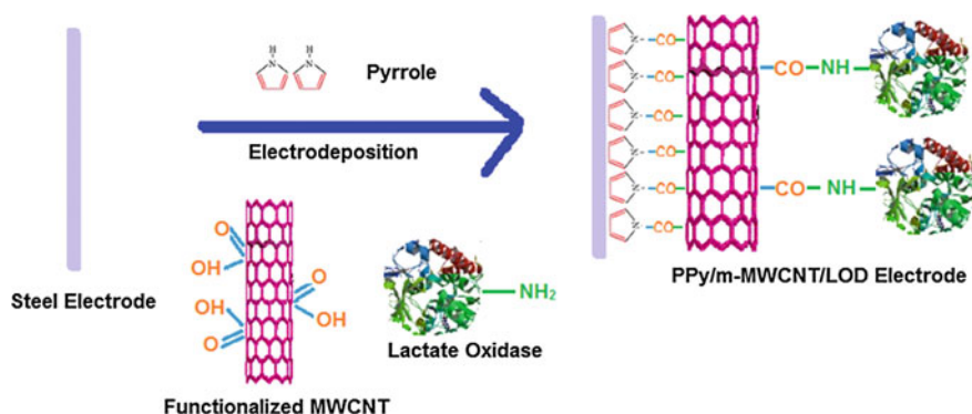
Fig. 23 Schematic diagram of the electrodeposition of PPy/c-MWCNT/LOD lactate biosensor
