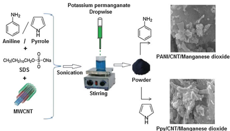
Fig. 27 Schematic illustration of preparation of PANI/CNT/MnO 2 and PPy/CNT/MnO 2 ternary nanocomposites
