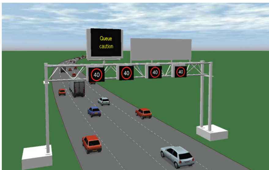
Fig. 4.17 VMS gantry controlled by ATM
