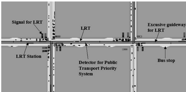
Fig. 3.32 An example of the LRT simulation with PTPS
