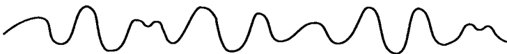
Figure 2.44. Recurring modulation and demodulation of the wave envelope (from Lake et al., 1977).
