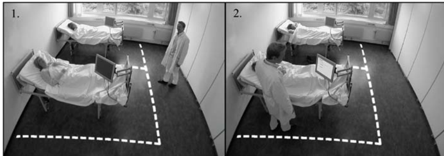
Figure 7. Fixed bedside terminals replace the mobile device used in the interaction design solution shown in Figure 6
