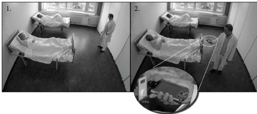
Figure 8. The location-aware zones surrounding each patient bed in Figures 6 and 7 are replaced by physical tokens (cards) containing bar codes. The tokens act as physical links to the patients' medical record. Scanning the barcode on a token with a mobile device retrieves the corresponding information
