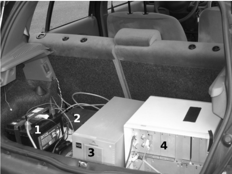
Figure 7.3. View of the rapid prototyping system placed in the booth. 1 Lead-acid battery powering the IBM TM compatible PC and the interface rack 2 General switch 3 IBM TM compatible PC 4 interface rack
