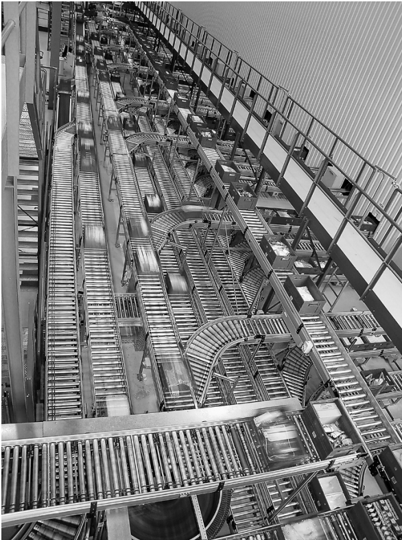
Fig. 4-140. Roller conveyors used in a logistics centre
