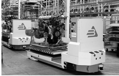
Fig. 4-20. Automated driverless transport system
