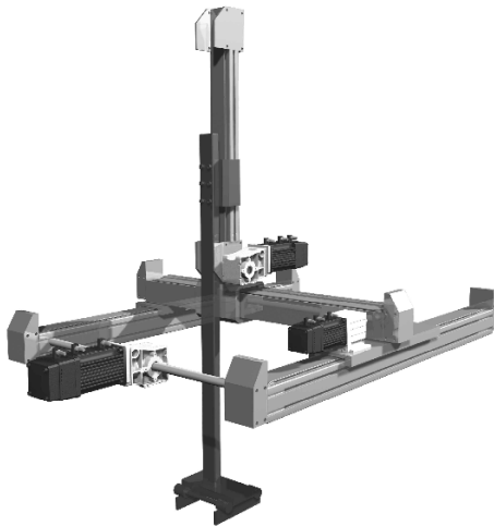
Fig. 4-57. Schematic diagram of a gantry robot or Cartesian robot
