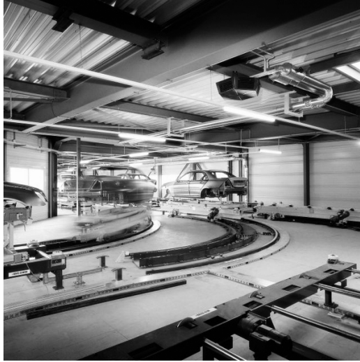
Fig. 4-18. Track vehicle system in the automotive industry
