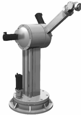
Fig. 4-61. Schematic diagram of a spherical robot
