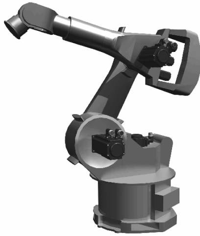
Fig. 4-59. Schematic diagram of a vertical articulated robot
