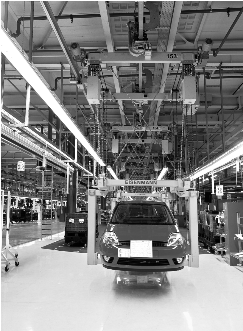
Fig. 4-36. Heavy-duty monorail overhead conveyor
