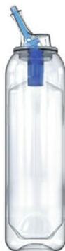
Fig 5.9 An overview of “bag-on-valve” (BOV) technology. The bag and valve are inserted into the canister during assembly. The canister is pressurized with the bag then filled with drug product (courtesy of Aptar Pharma)
