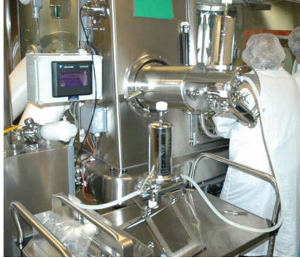
Fig. 9.6 Stainless steel transfer system for liquid (courtesy from Getinge La Calhène)
