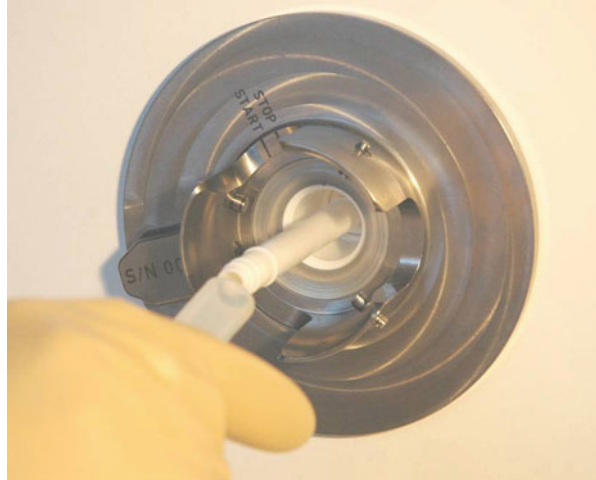
Fig. 9.5 Silicone tubing connection to a SART connector placed inside its RTP
