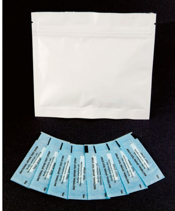
Fig. 18.1 An example of a biological indicator used for a heat sterilization validation. Photo courtesy of Mesa Laboratories, Inc
