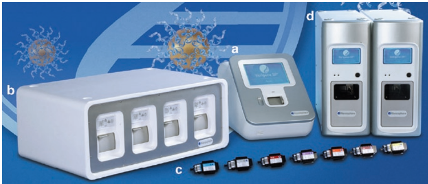
Fig. 2.4 The Verigene™ genotyping platform. (a) The Verigene Reader is barcode scanning and network communication-enabled central control unit and main user interface. (b) The Verigene Processor is comprised of four independent test modules controlled by the Verigene Reader. It facilitates the wet chemistry inside the test cartridge (c). Test processing in this module relies on offline nucleic acid extraction. (d) The Verigene Processor SP possesses all of the same test processing functionality and components as the regular processor but additionally provides capabilities to extract DNA directly from the specimen. These additional functions require the following consumables: a Verigene Extraction Tray and Verigene Tip Holder Assembly (not shown). (Courtesy of Nanosphere)
