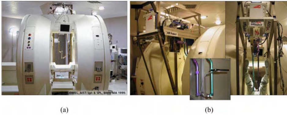
Figure 2. (a) GE Signa SP open-MRI scanner, with (b) integrated 5-DOF MR-compatible robot. The robot end-effector is equipped with an optical tracking marker (inset).
