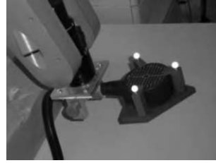
Figure 4. Calibrating the robot mounted TMS coil using POLARIS and KUKA position information. The calibration tool will be removed during treatment.
