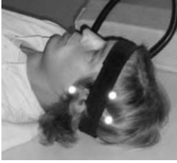
Figure 3. Tracking the head by attaching a headband with POLARIS markers to it. All points acquired during registration are referenced to the headband coordinate system.
