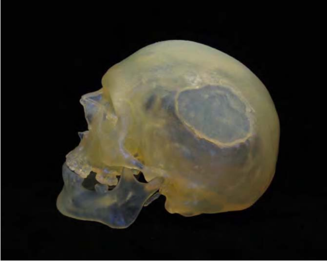
Figure 5. Stereolithography fabricated skull with implant in place.
