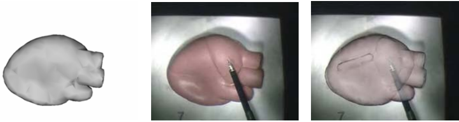
Figure 1. Illustrations of the 3D reconstruction model, the first video frame in the sequence and the overlay of the 3D model registered with the video frame.
