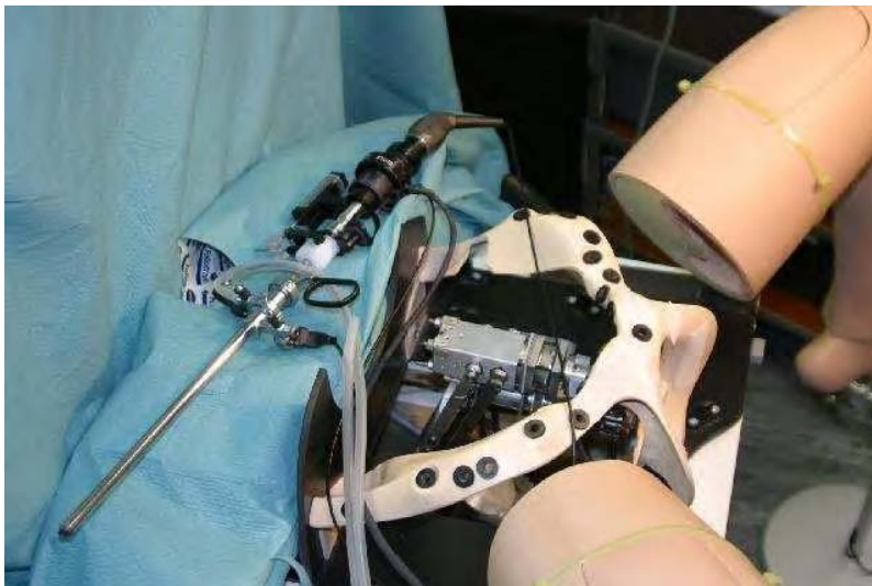
Figure 2. Haptic mechanism inside dummy.
