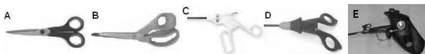
Fig. 4 A. Pair of household scissors; B. Pair of material shears; C. Autosuture EndoShears Pistol Grip Handle Laparoscopic Scissors; D. Karl Storz 33124 Inline Handle Laparoscopic Scissors; E. Karl Storz Endoskope multifunctional handle.
