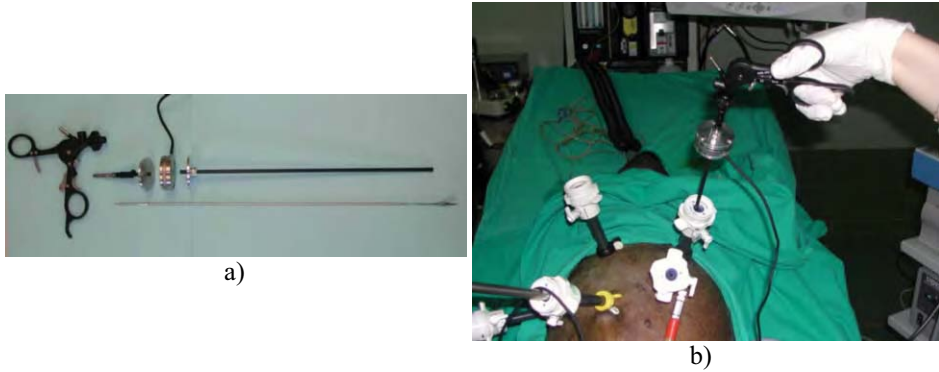
Figure 1: Device designed to acquire laparoscopic interaction forces. a) Device dismantled in its different components: the black tube has been cut and two metal plates have been designed to fix the F/T sensor. The metal axis is introduced in the black tube and is responsible for the transmission of the grasping movements. b) Device being used in the pig model through a trocar in the forces measurement study.
