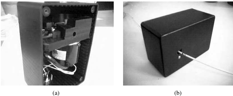
Figure 1. The catheter tracking device. (a) Rotary encoder, (b) The assembled device. A catheter can be seen passing through it.
