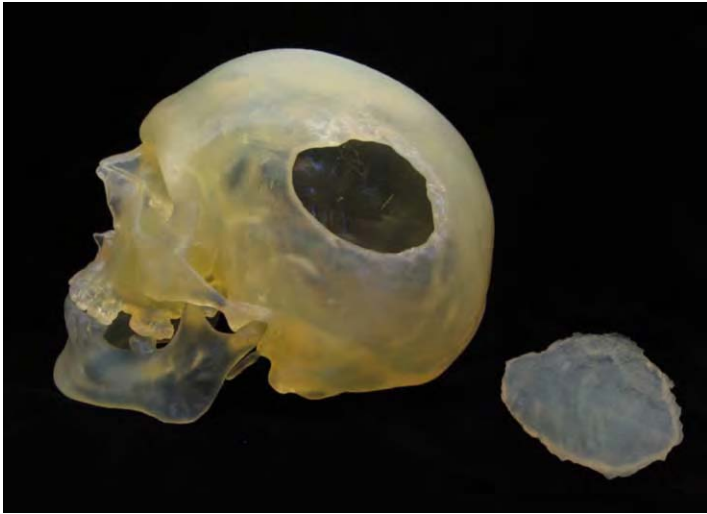
Figure 4. Stereolithography fabricated skull with a simulated defect and the implant.
