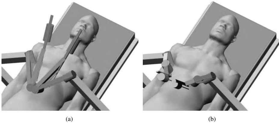
Figure 1. (a) Robot arms with long ( 90^\circ , 90^\circ ) links suffer from elbow collisions when performing tasks such as running the bowel. (b) Robot arms with short ( 39^\circ , 33^\circ ) links suffer from kinematic singularities at the workspace boundary.
