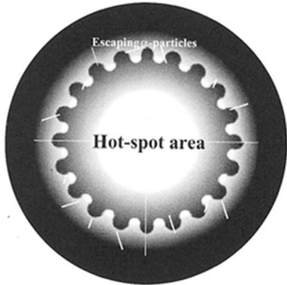
Fig. 3.27 Depiction of the reduced self-heating of the hot-spot area from prematurely escaping \alpha -particles
