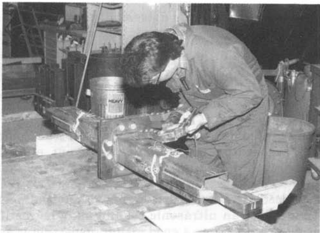
FIGURE 8.23 Magnetic particle inspection of a connection (University of Toronto)
