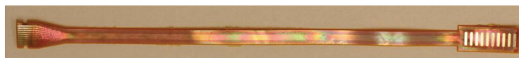
Figure 1.5 Amorphous SiC (a-SiC) coatings are readily formed using various processes such as RF sputtering, PLD, plasma spraying, etc. These coatings can be realized at low temperatures thus allowing for the coating of soft, low-temperature materials such as polymers and plastics. Photo shows an a -SiC-coated polyimide brain-machine interface (BMI) device. (Photo courtesy of A. Hess et al. [67].)
