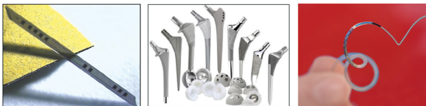
Figure 1.7 Reported SiC biomedical devices. From left to right, myocardial heart probe [43], bone prosthetic [76], and coronary heart stent [77]. The heart probe is made of single-crystal bulk 6H-SiC, while the bone prosthetic is SiC-coated titanium to eliminate ion uptake in the body. The heart stent is SiC coated to greatly reduce clotting and thus eliminate the need to perform a second surgery to replace the stent. (Photo courtesy of Christoph Hehrlein [78].)
