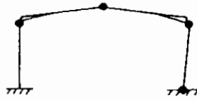
Fig. 11.11 Basic collapse mechanism (Mode 1) for haunched portal.
