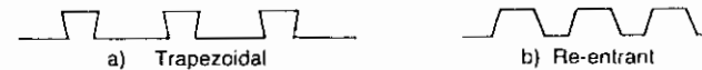
Fig. 9.14 Typical profiles—various depths, various forms of indentation and various types of stiffening are used.
