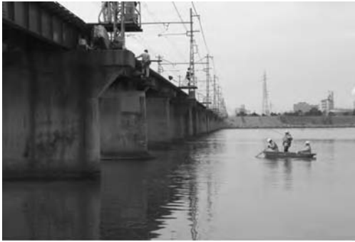
Figure 6. Impact vibration test.
