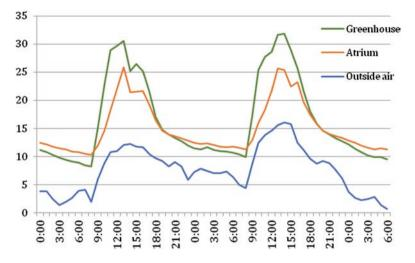
Fig. 3 Time course of ICTA greenhouse, atrium and outside air temperature, days 24–25 January 2015. Greenhouse without plants (Source: Montero et al. 2016)
