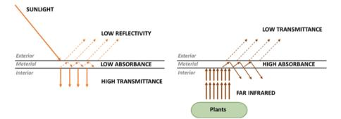
Fig. 2 Desired behaviour of materials against sunlight (*left*) and far infrared (FIR) (*right*) to maximize crop yields (Source: E. Sanyé-Mengual, J.I. Montero)
