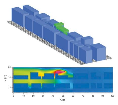
Fig. 2 Top, a sketch of the street canyon with the green roof and bottom, the air temperature differences (Image. T.Georgiadis)
