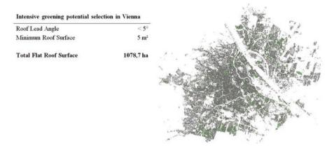
Fig. 4 Flat roofs identification and mapping with ARCGIS (Source: Dang 2016)
