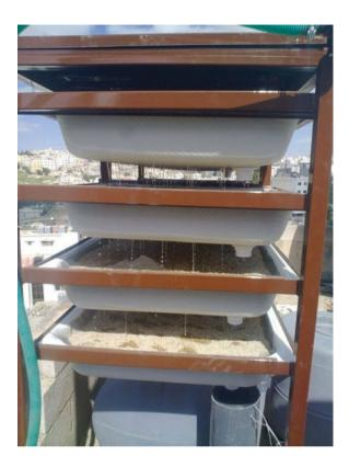
Fig. 4 The new greywaterrecycling unit (Credit: Heshem el Omari)
