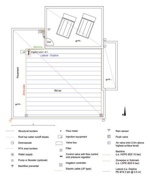
Fig. 1 Sample of a micro-irrigation system layout for rooftop agriculture
