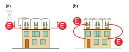
Fig. 1 Energy flows in isolated rooftop greenhouses (open-cycle) and integrated rooftop greenhouses (closed-cycle) (a) Isolated RTG, (b) Inegrated RTG (Image: E. Sanyé-Mengual)
