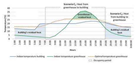
Fig. 4 Graphical representation of residual heat in RTG-Building system (Source: Cerón Palma 2012)
