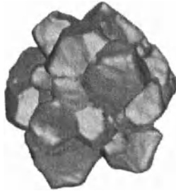
Figure 12. 37 grains of the 3D reconstruction data imported in the vertex dynamics model.
