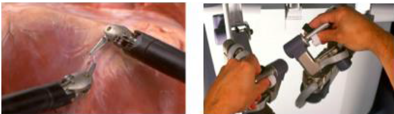
Figure 5-2 The robot arm (left) and operation manipulation (right) of Da Vinci surgical system. Source: [14] with permission, ©2014 Intuitive Surgical, Inc.
