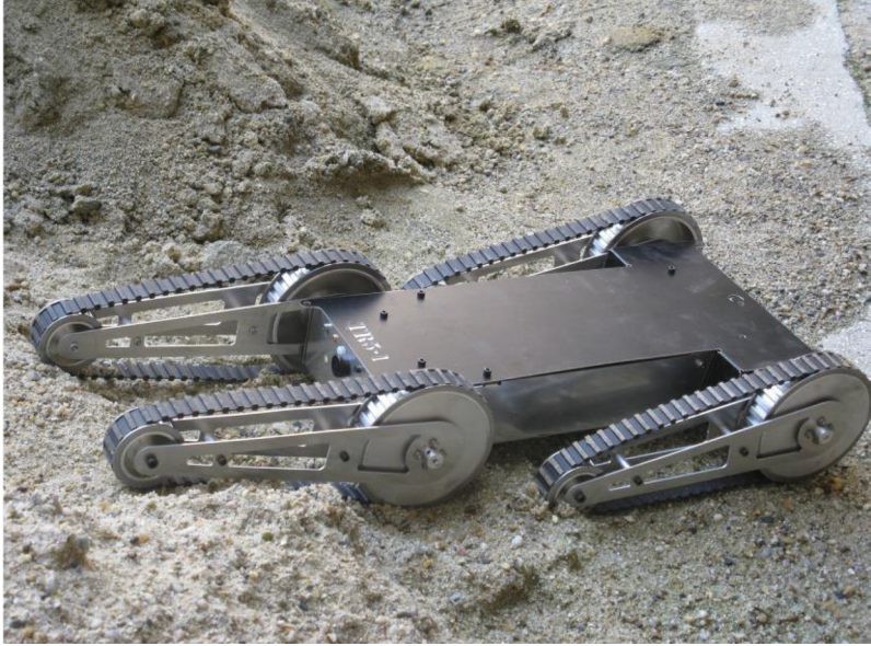
Figure 3-4 Testing of the climbing ability on soft terrain.
