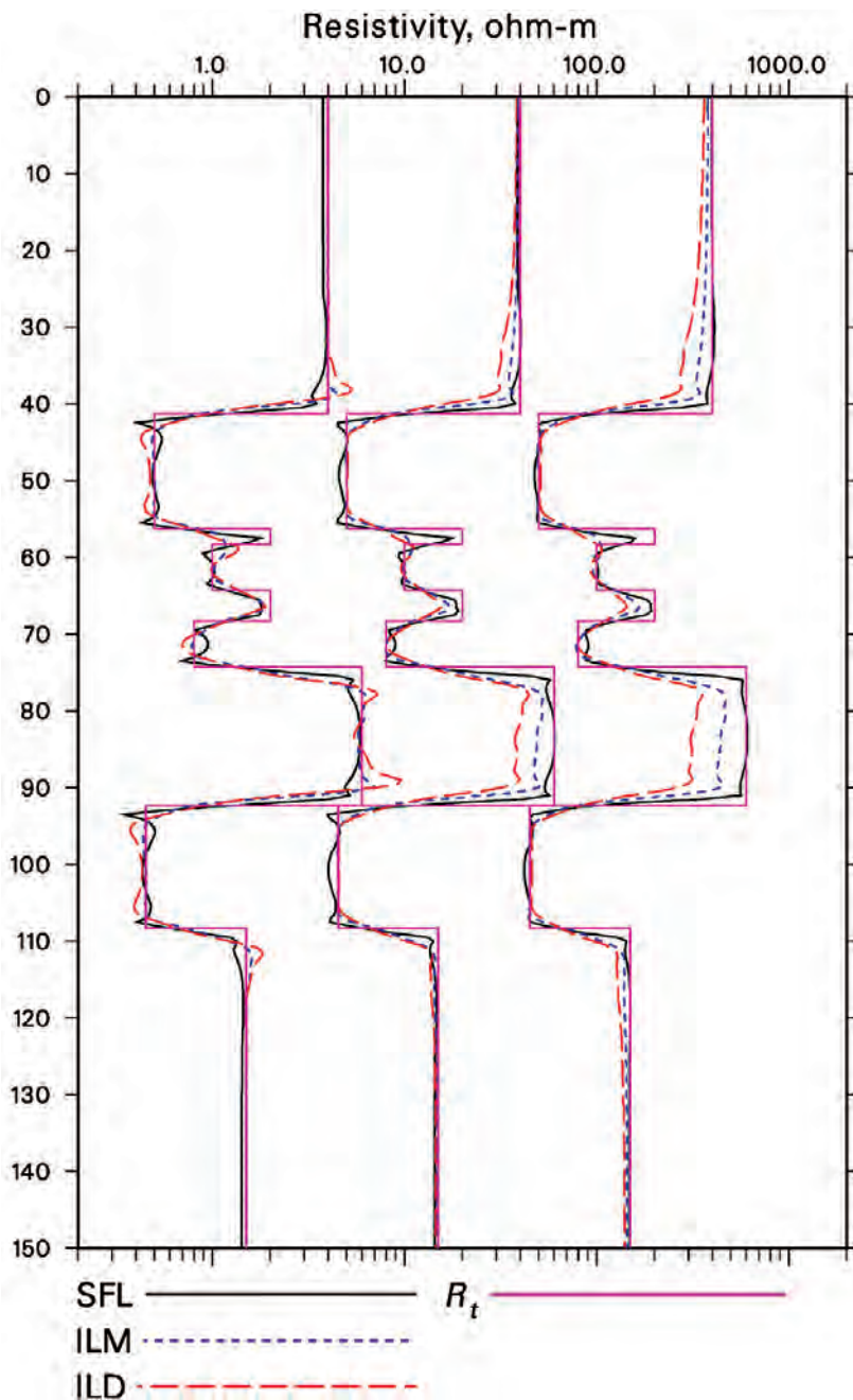
Fig. 3B.18—Modeled DIT logs in a set of formation layers with the same shoulder-bed contrasts, but centered on 1, 10, and 100 ohm-m.
