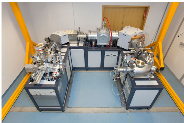
Fig. 4 MICADAS: AMS machine made by Ionplus AG and installed at the Royal Institute for Cultural Heritage, Brussels. ©KIK-IRPA
