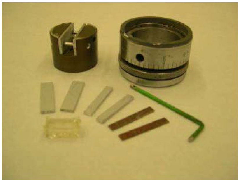
Fig. 7 Polishing sample holder. Reprinted from [56], with permission from Springer
