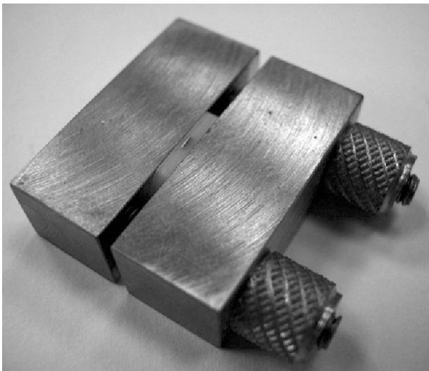
Fig. 4 Sample holder for samples embedded in a KBr pellet. Reprinted from [55], with permission from Elsevier
