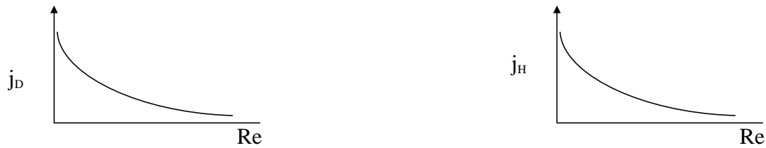
Figure 6.10 Sketches showing the variation of the mass flux j_D and heat flux j_H as a function of the Reynolds number, Re .
