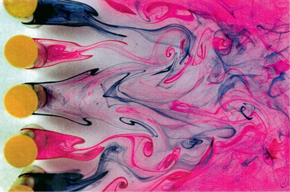
Figure 1.14. Flow past a grating of five circular cylinders visualized by two colours, by Tetsuo SAGA, The University of Tokyo, *Fantasy of Flow* (1993), by permission Ohmsha, Ltd
