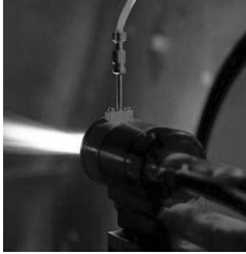
Figure 5.1 A Praxair SG-100 plasma spray torch in operation
